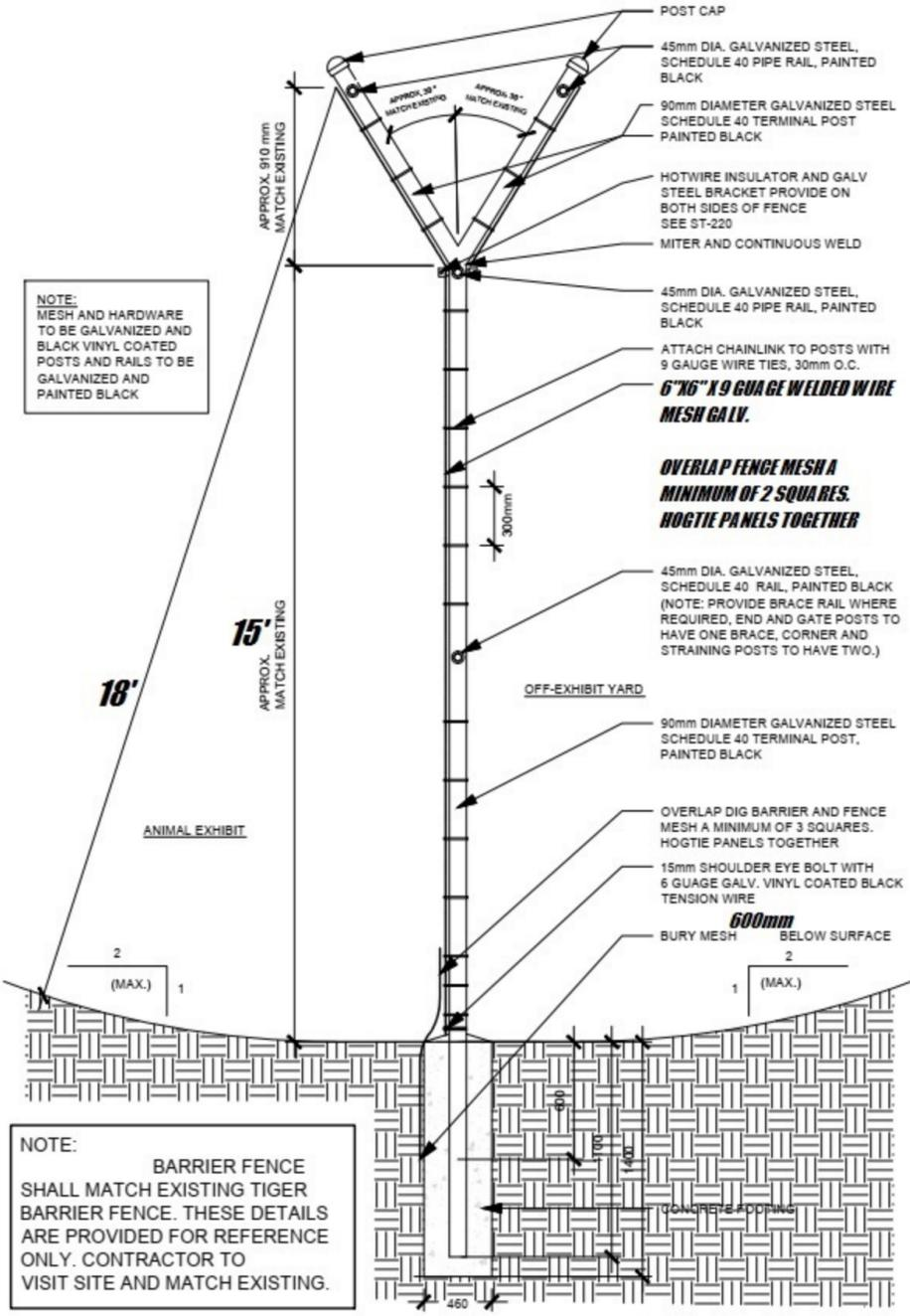
**16' High Barrier Fence W/ Double Outrigger Section**
