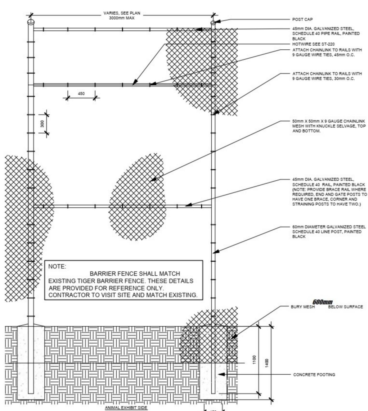
**18' High Barrier Fence Elevation**
