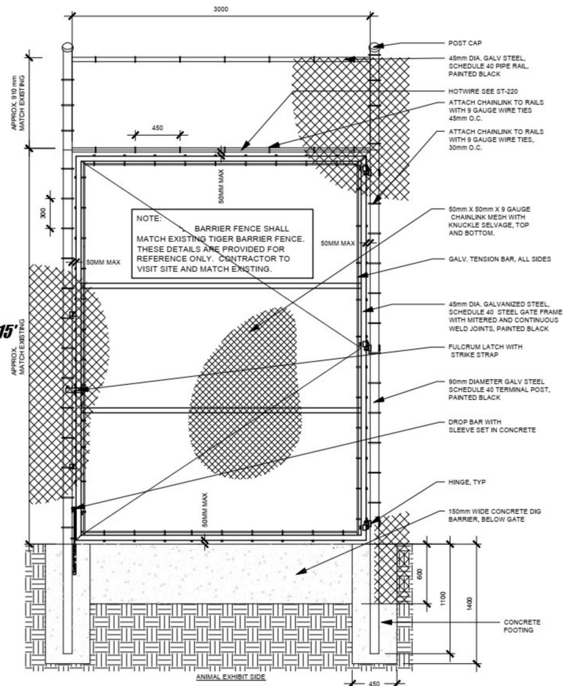
**Barrier Fence Gate Elevation**
